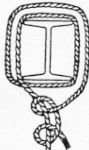
Bad Practice— Steel can cut rope
