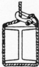
Bad Practice— Can bend flanges and cut rope
