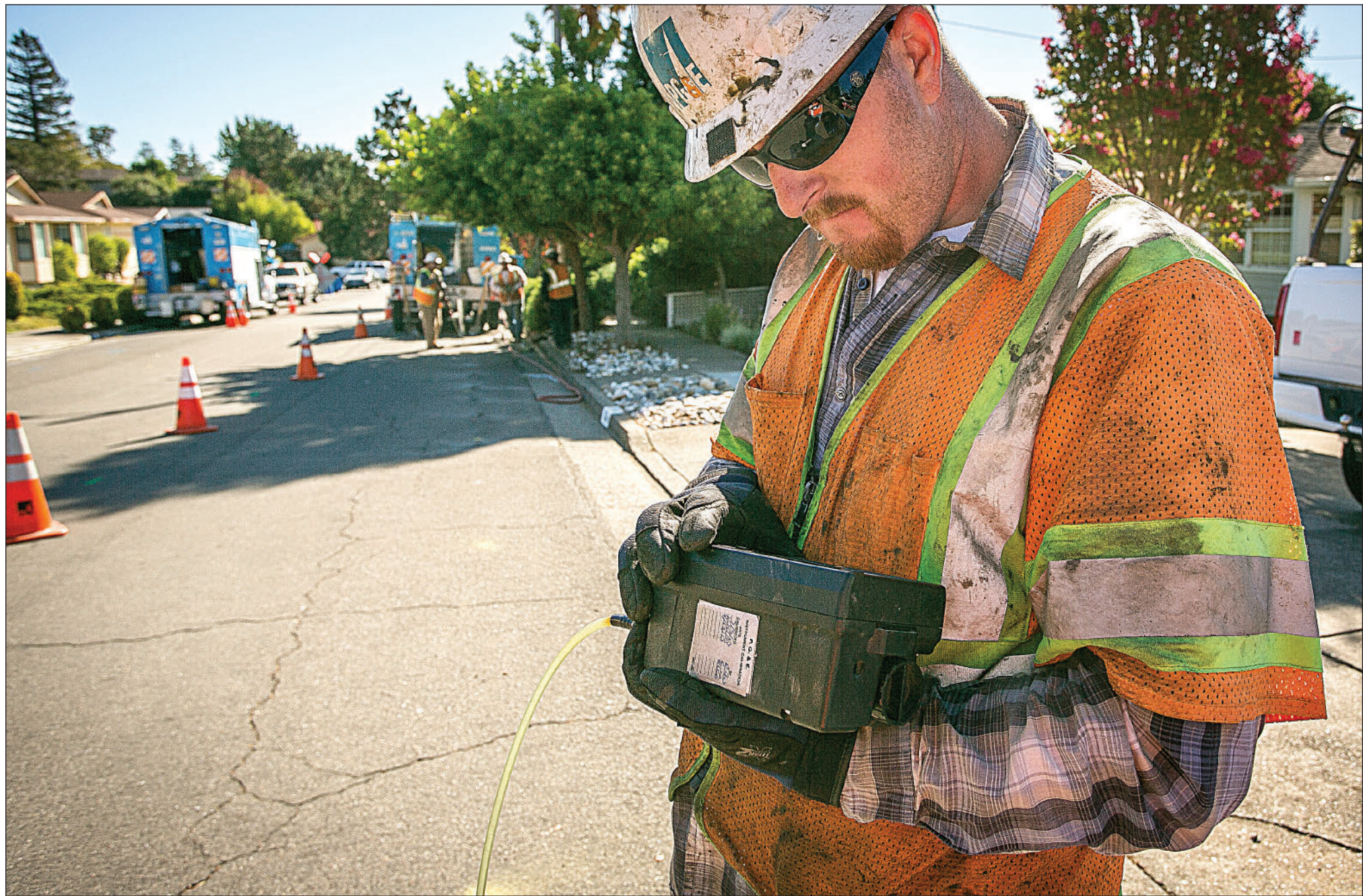
Josh Wisdom uses a combustible gas indicator to determine the amount of gas present in the hole.
