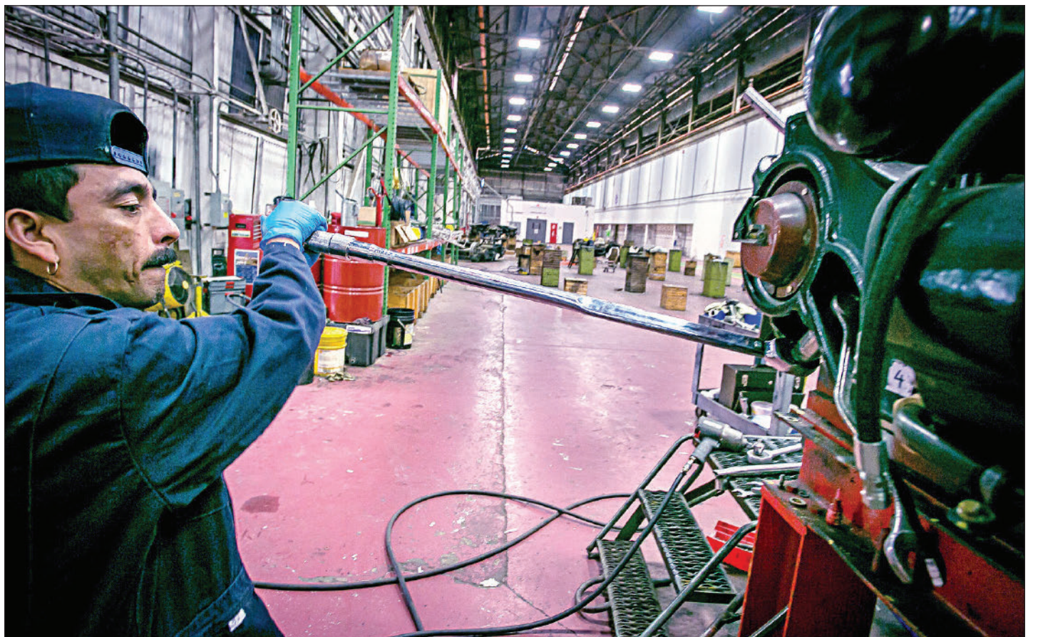
Mechanic Rodolfo Nunez, shown here and above, is torquing the bolts to the primary suspension on the trucks (axles).
