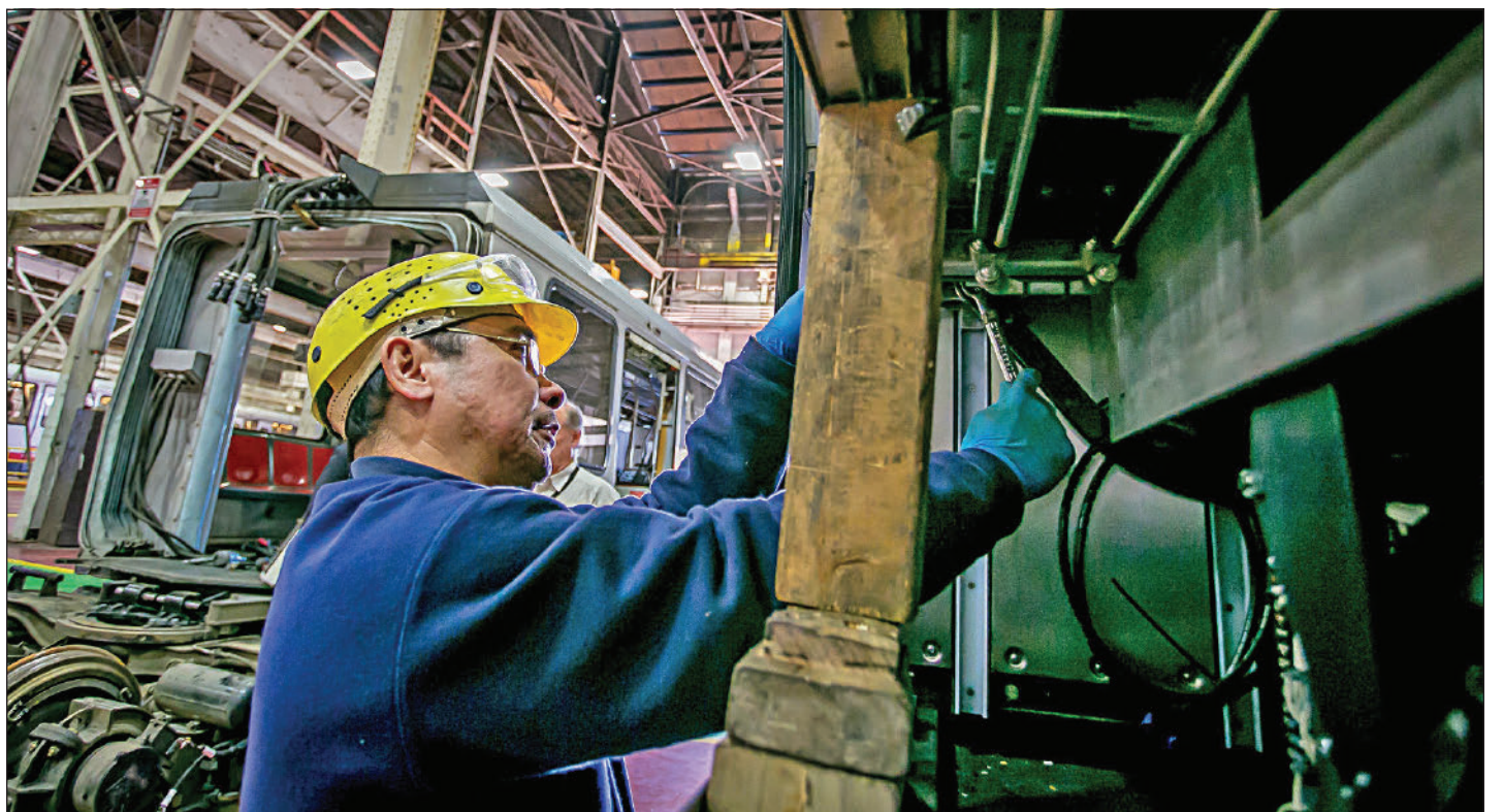
Mechanic Jose Morente is testing and adjusting the hydraulics for steps.
