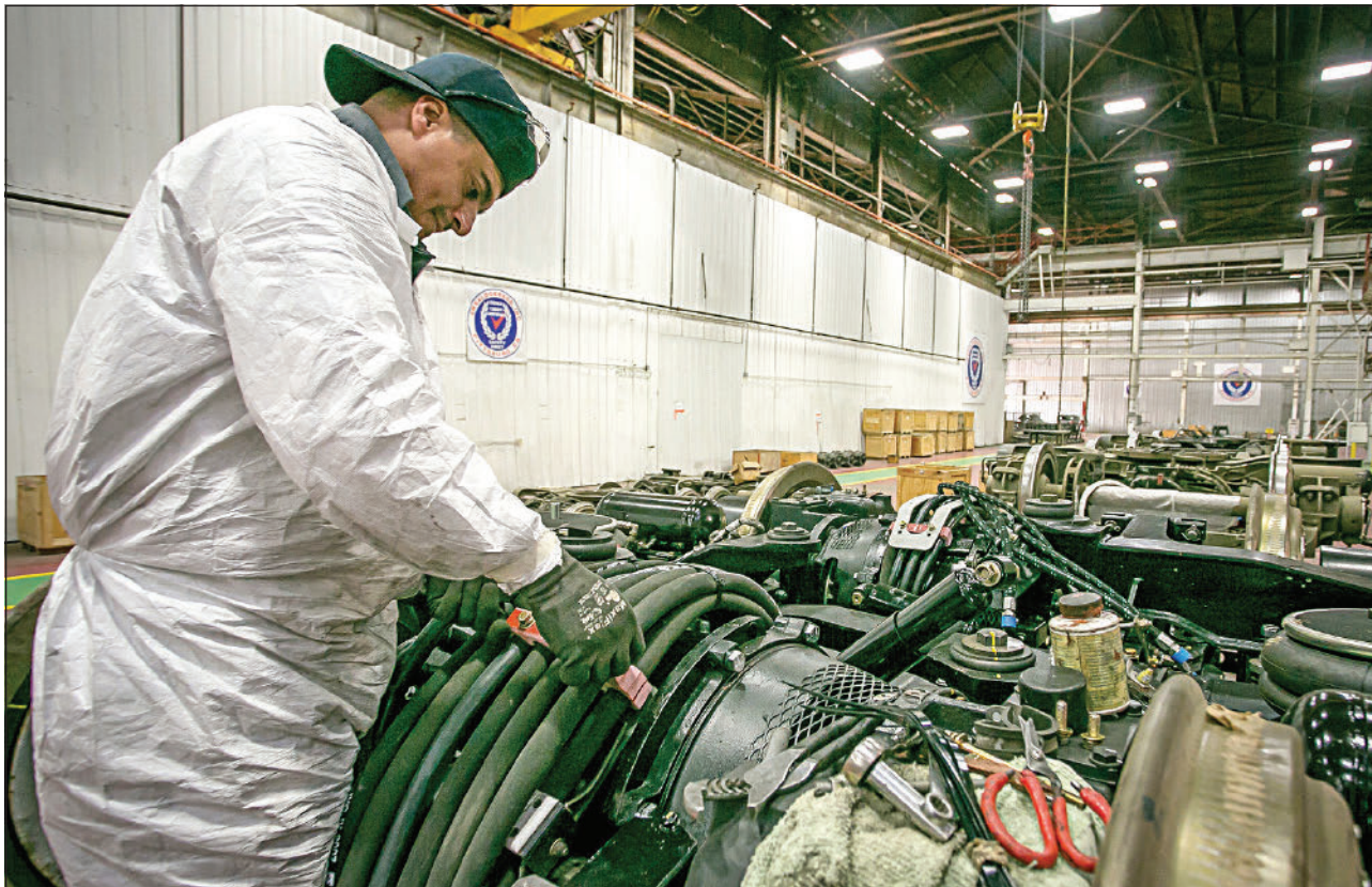
Lead Mechanic Miguel Perez is installing new cables for the new motors on the trucks. Photos by John Storey
