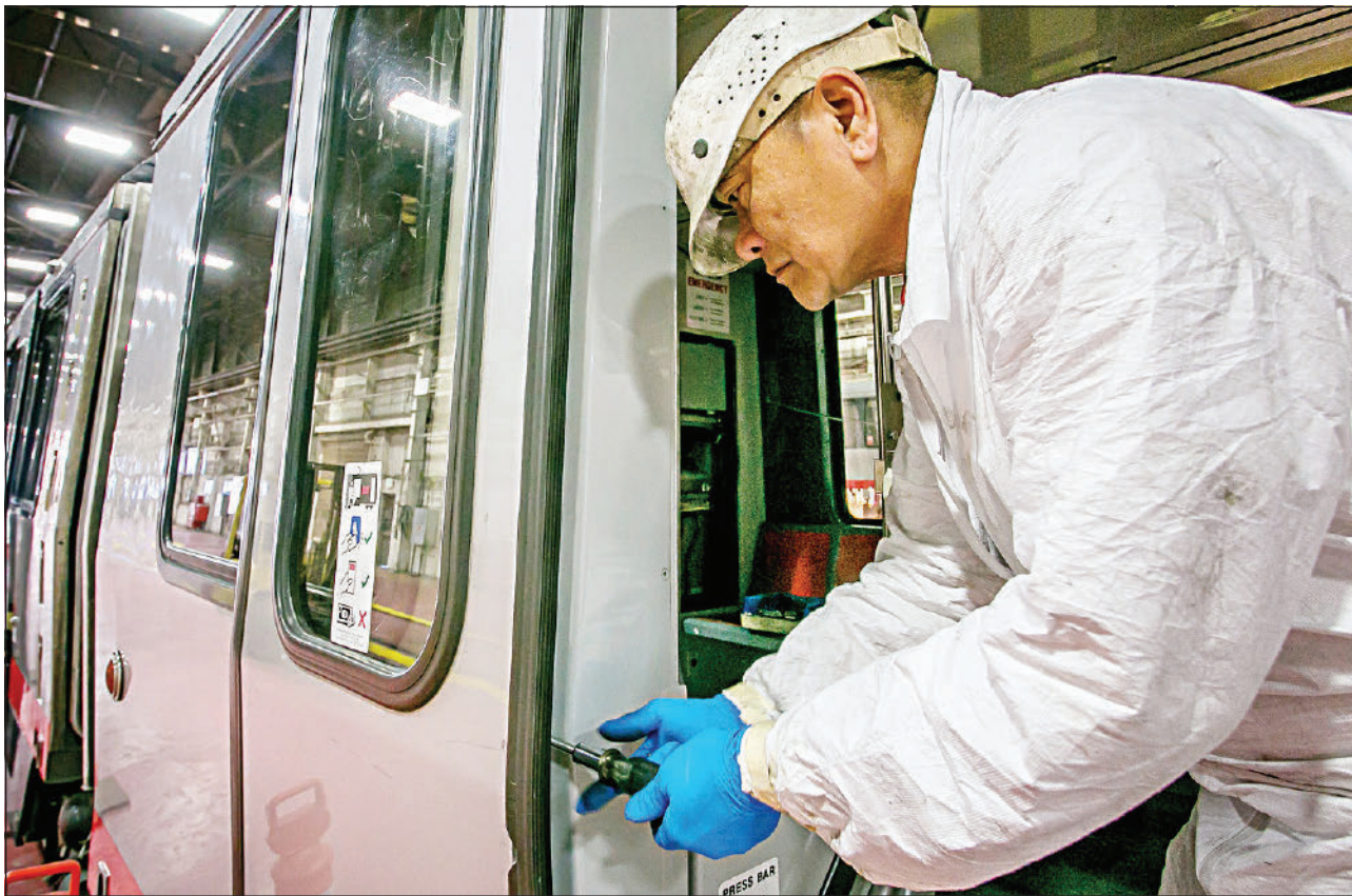
Mechanic Nicasio Blanco is installing the Ekart covers that control the opening and closing of the doors.
