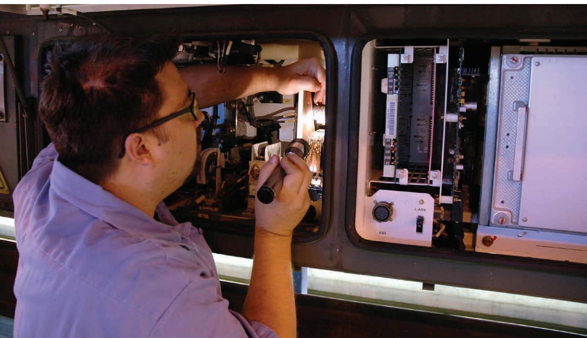
Brian Medeiros, an "A" Mechanic, inspects the main contactor for the LRV's propulsion system.
