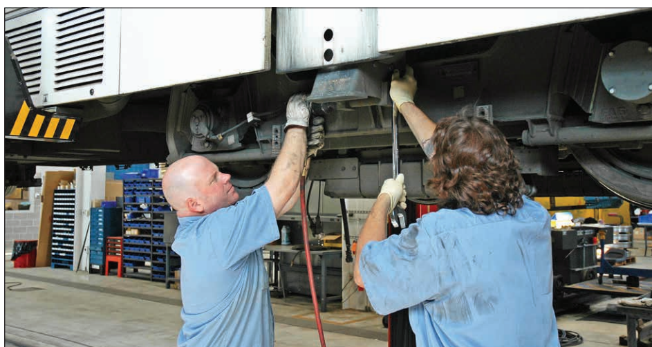
Matt Mibach, left, and Robert Bonsack, both "A" Mechanics, adjust bolts holding the bus to the truck. They are replacing the truck with one that's been serviced.
