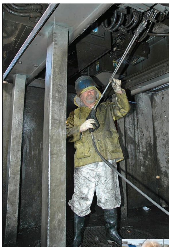
"C" Mechanic Gary Rice hoses down the underside of a light rail vehicle so that it can be inspected.
