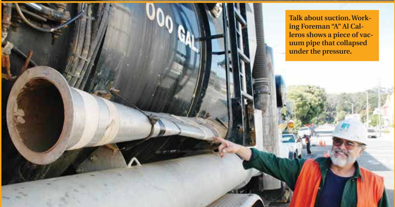
Talk about suction. Working Foreman "A" Al Calleros shows a piece of vacuum pipe that collapsed under the pressure.
