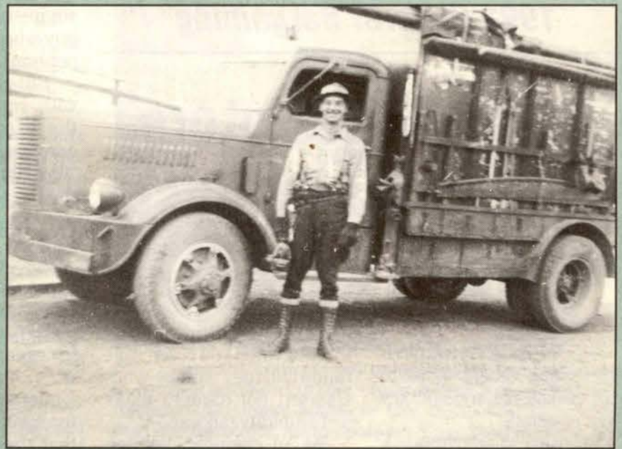
Pat Patteson with one of the "better line trucks for those days" (about 1948 in Hayfork, Ca.). Says Patteson today: "They sent us stake side trucks and built them into line trucks on the job as we worked. This is an old FWD. In the snow they could sure break roads in the snow to help people get to the highways to get to the doctor or hospital." (Courtesy C. L. Patteson)
