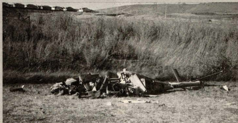
Close-up of helicopter which crashed after contacting 230kv power line at the Exxon refinery. A power outage resulted in the surrounding area.
