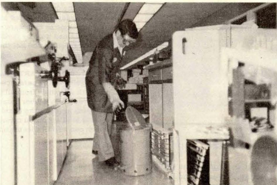
A foot-controlled disposal can was recently introduced in Reprographics so that solvent contaminated rags can be discarded immediately after each use. Frequent disposal reduces unnecessary solvent evaporation into the workplace atmosphere.
