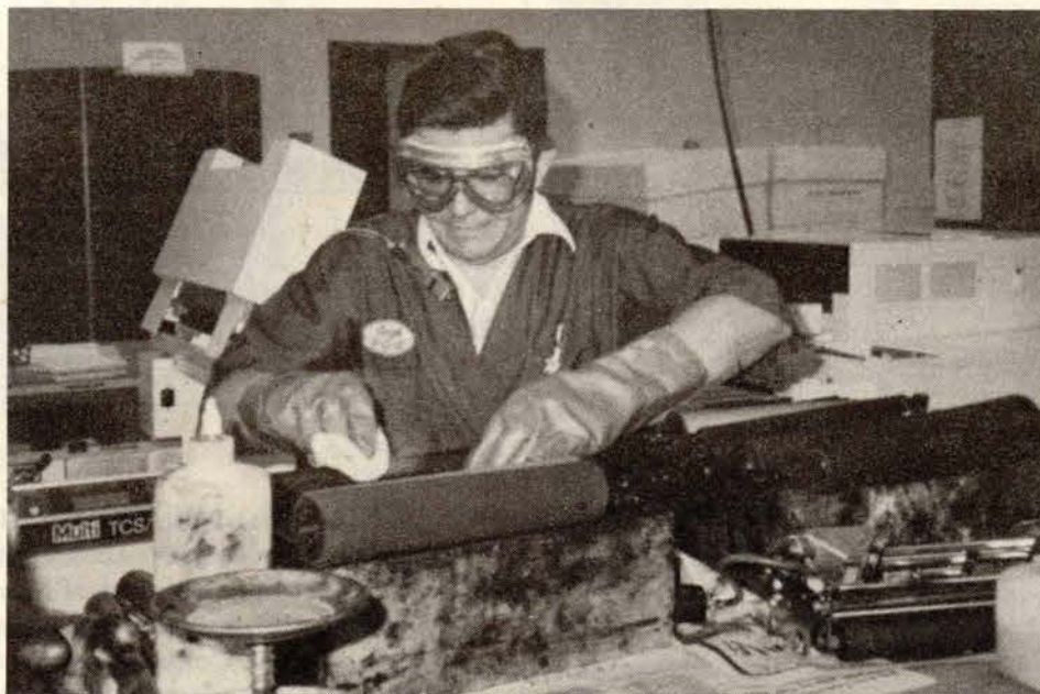
Angel Alvira, Operator A and member of IBEW Local 1245, uses the new work practice methods while removing ink from the rollers of a large printing machine. A charcoal-filled glass tube is clipped to his lapel. The charcoal tube, which is connected in series to a portable pump, is used to collect hazardous breathing zone vapors to be measured later by a chemical laboratory.
