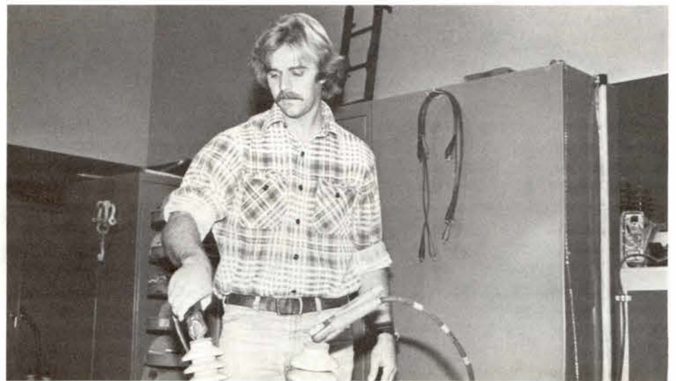
Senior Meterman Gary Fromm tests a transformer brought in from the field by energizing the transformer at the primary voltage.
