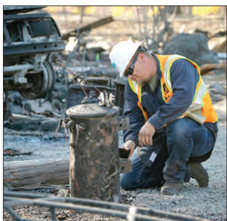
Scott Schweikl uses his phone to take a photo of a burned transformer.
