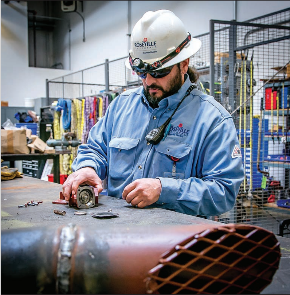
Mechanic Guadalupe Oseguera rebuilds a pump in the power plant maintenance room.
