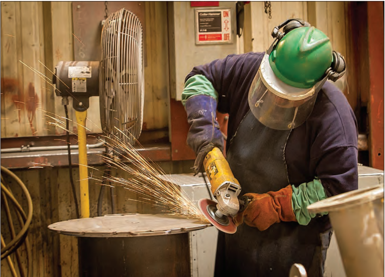
Hugo Montellanos buffs the edge of a transformer piece
