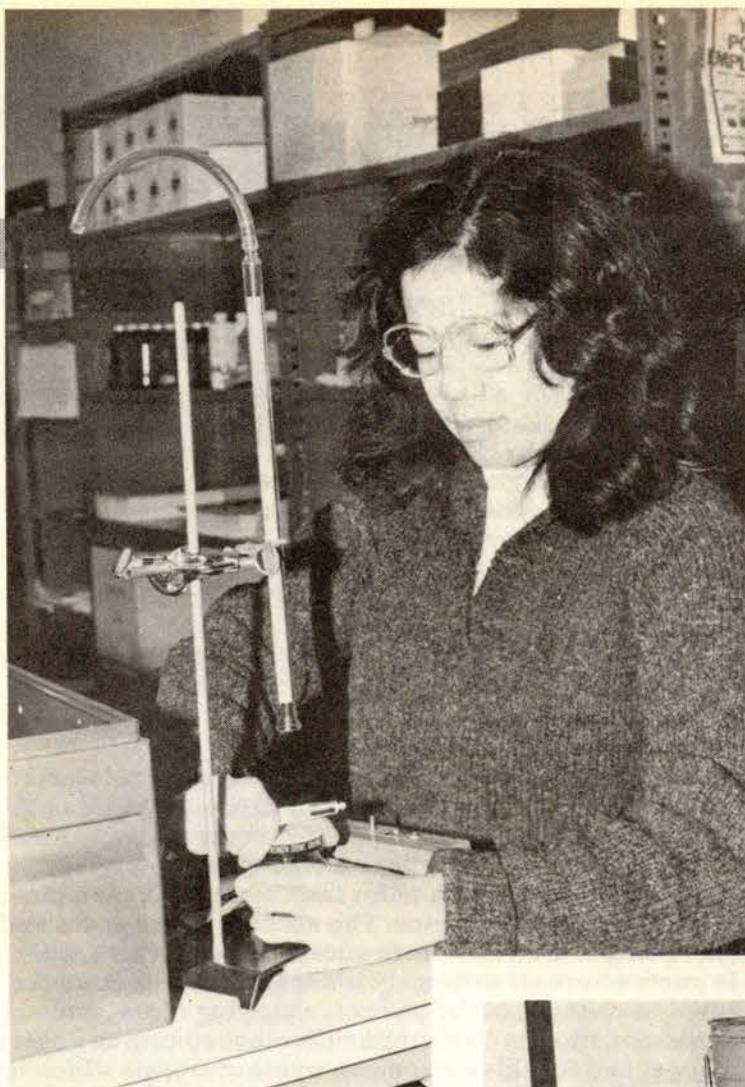
Sum opens jar of soapy water which is used in the bubble meter system.
