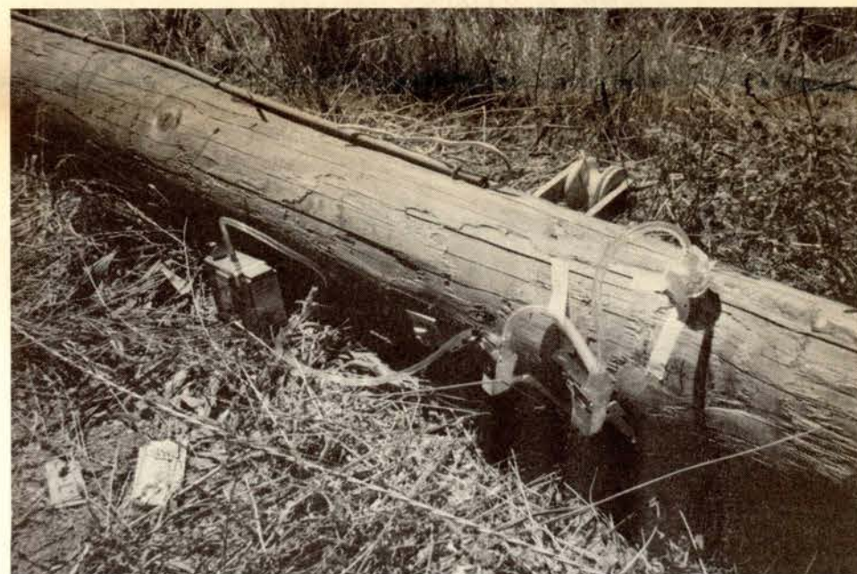
After Gilbert, above, drilled hole, monitoring equipment was then placed at the newly drilled hole to collect pentachlorophenol gases and vapors. This equipment includes a filter, 2 flasks containing ethylene glycol, and a high flow pump.
