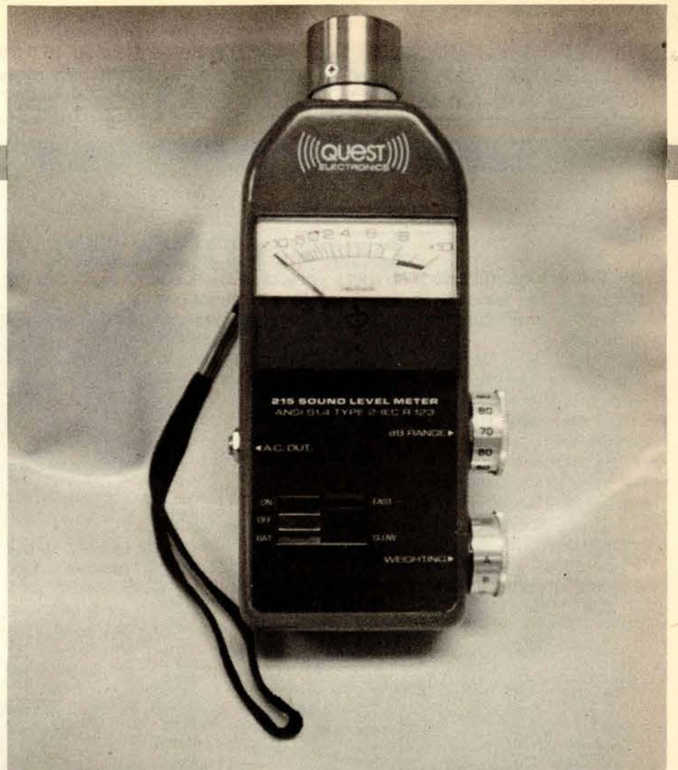
Meter used by Local 1245's Industrial Hygienist Juliann Sum to monitor safe and hazardous noise ranges on the job.
