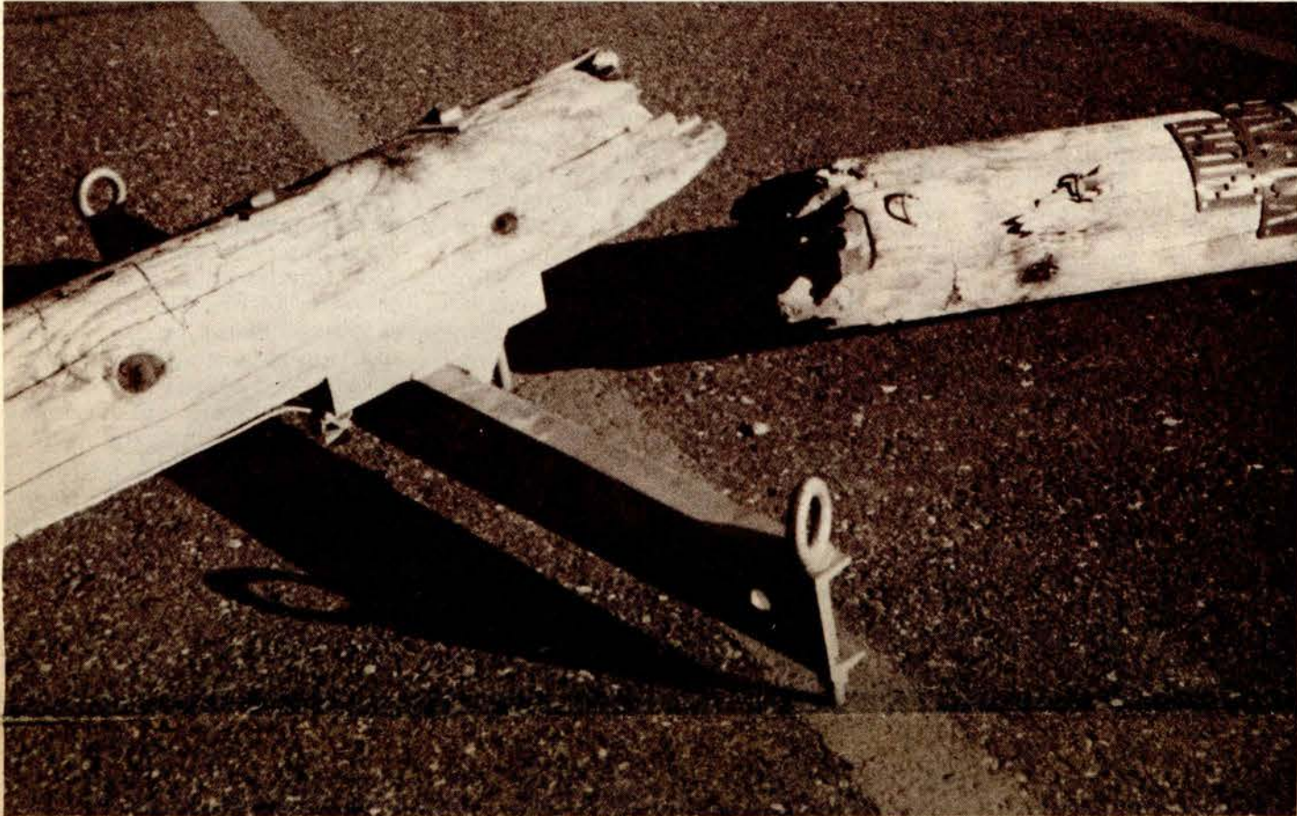
Photo shows graphic reality of unexplained pole break in San Luis Obispo area where a hazard alert has been issued. No injury was related to the incident.
