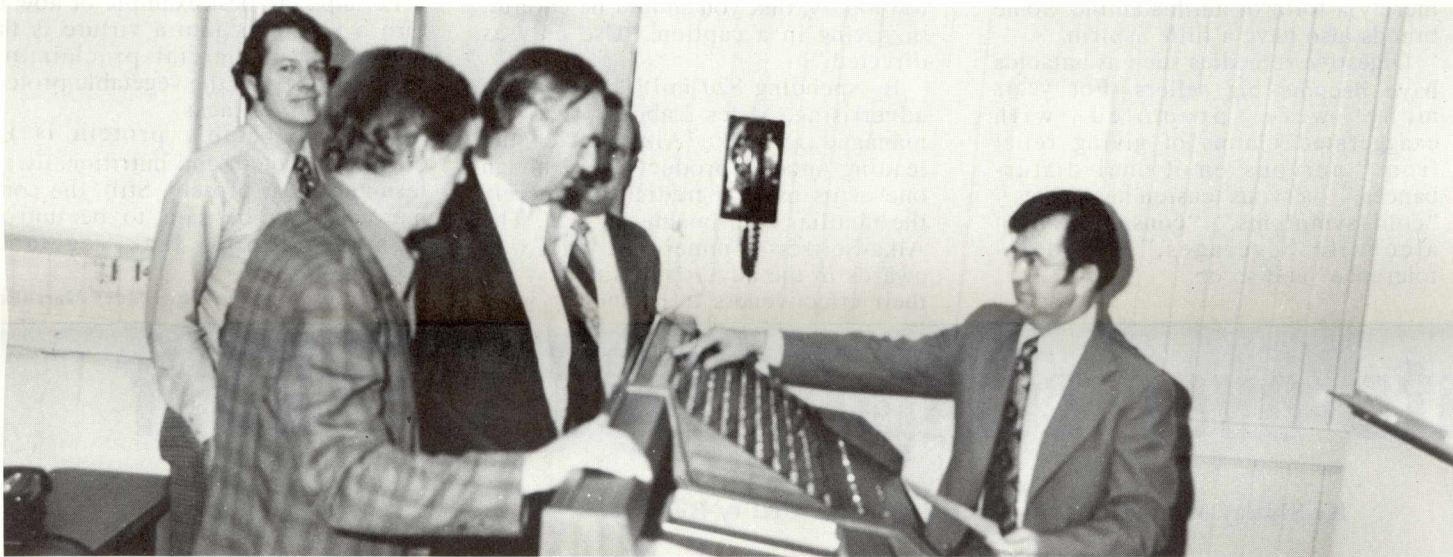
This picture shows Don Davis at the Simulator Master Console. At the Console, trouble can be set up anywhere in the Simulated system. The console has the capability, through five different timers, to set cascading trouble in the system.
