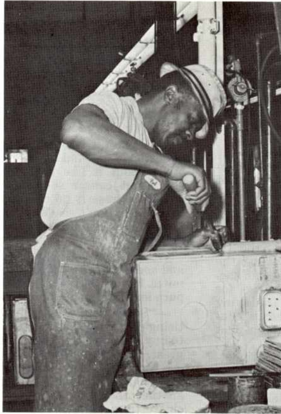
The above photo shows Wally Hunter, Meter Shopman, repairing a 5-B tin meter at the Gas Meter shop.
