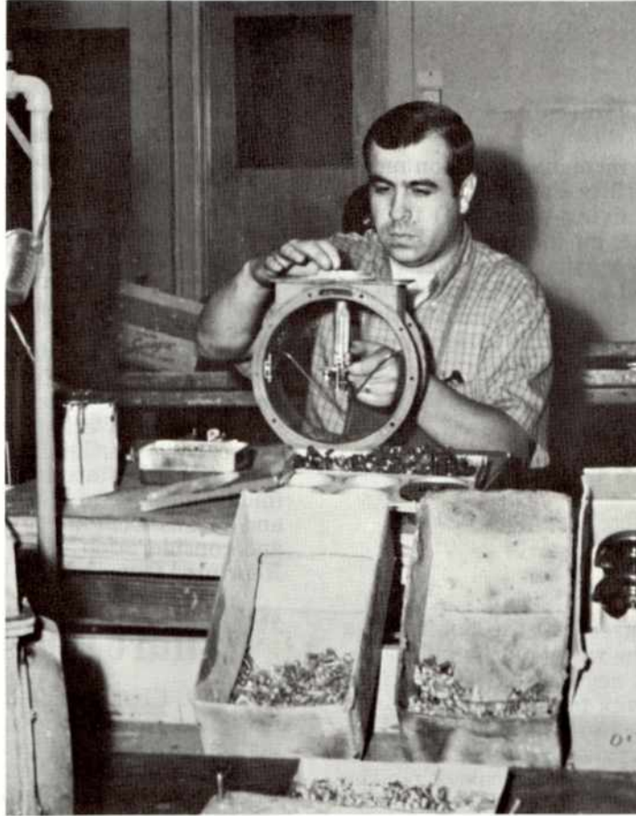
John Musgrove, meter shopman and Shop Steward in the Gas Meter Shop, is shown repairing a gas meter.
