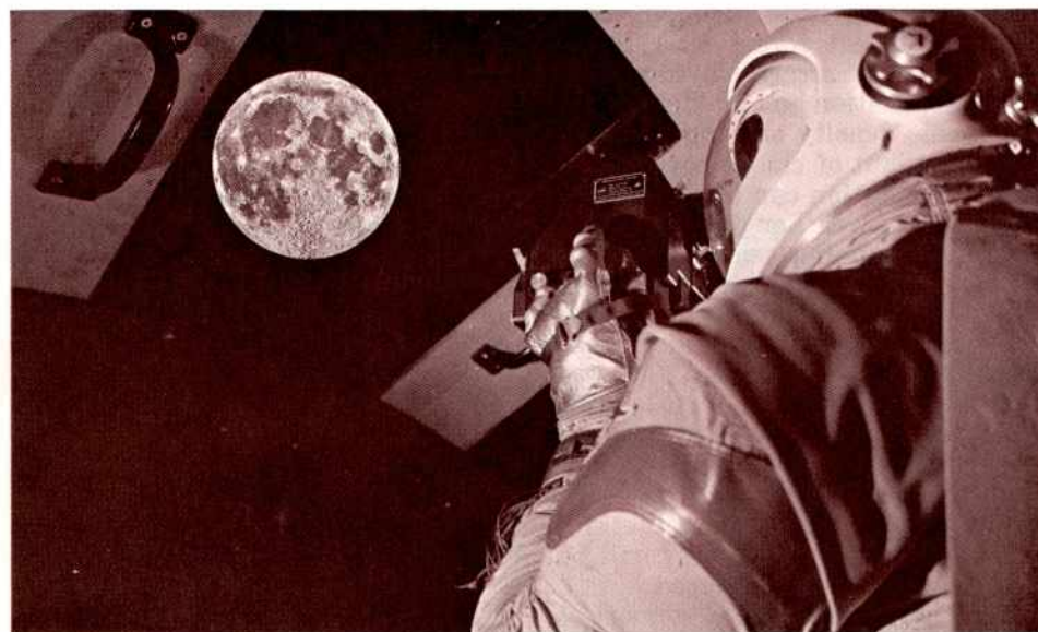
A research scientist is seen here using a "Space Sextant." It is used to measure the angles between two objects in navigation. He is seen sitting in a laboratory model of the Apollo space vehicle and looking at a simulated moon.
