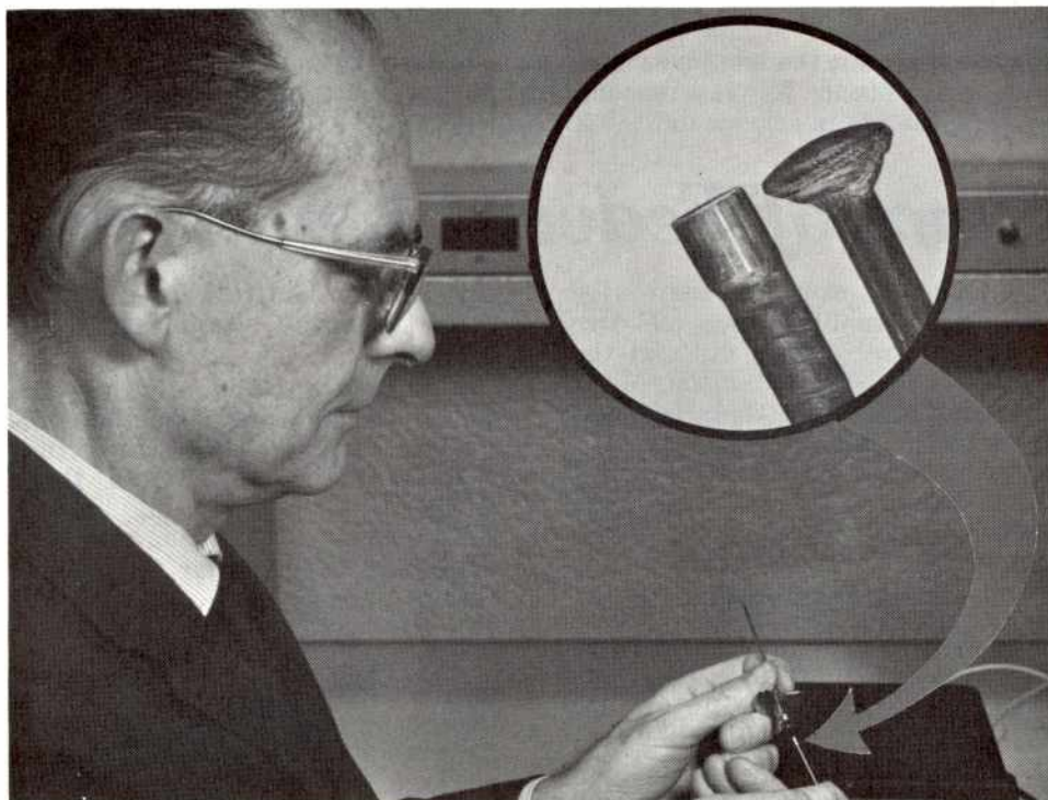
An extremely small blood pressure sensor is shown here (inset) next to the head of a pin. It can be inserted into blood vessels through a standard hypodermic needle.
