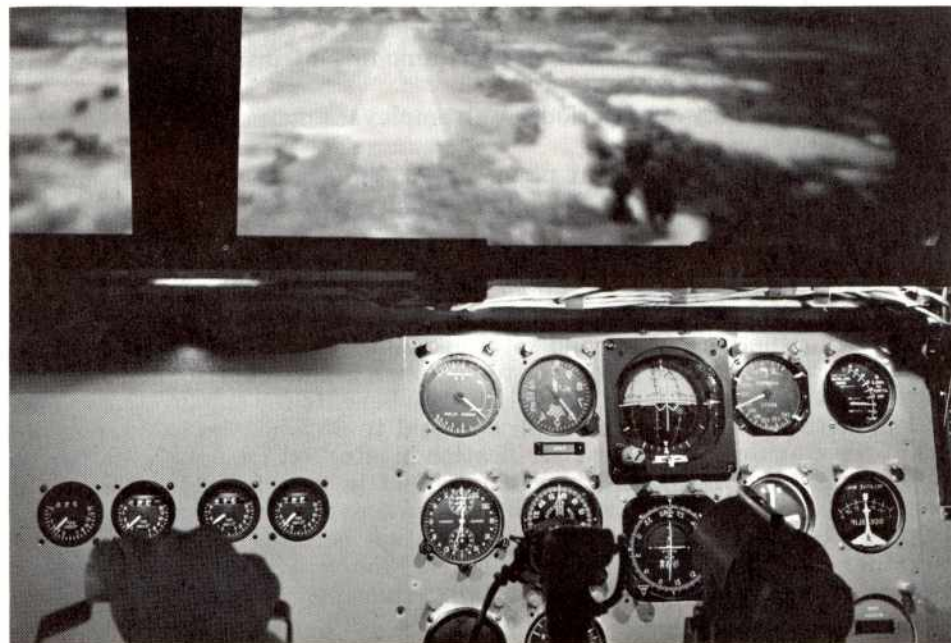
A simulated airport runway is seen here by pilots practicing landings in a NASA flight simulator. The sights and sounds of a DC-8 jet aircraft can be duplicated accurately in this test facility.
