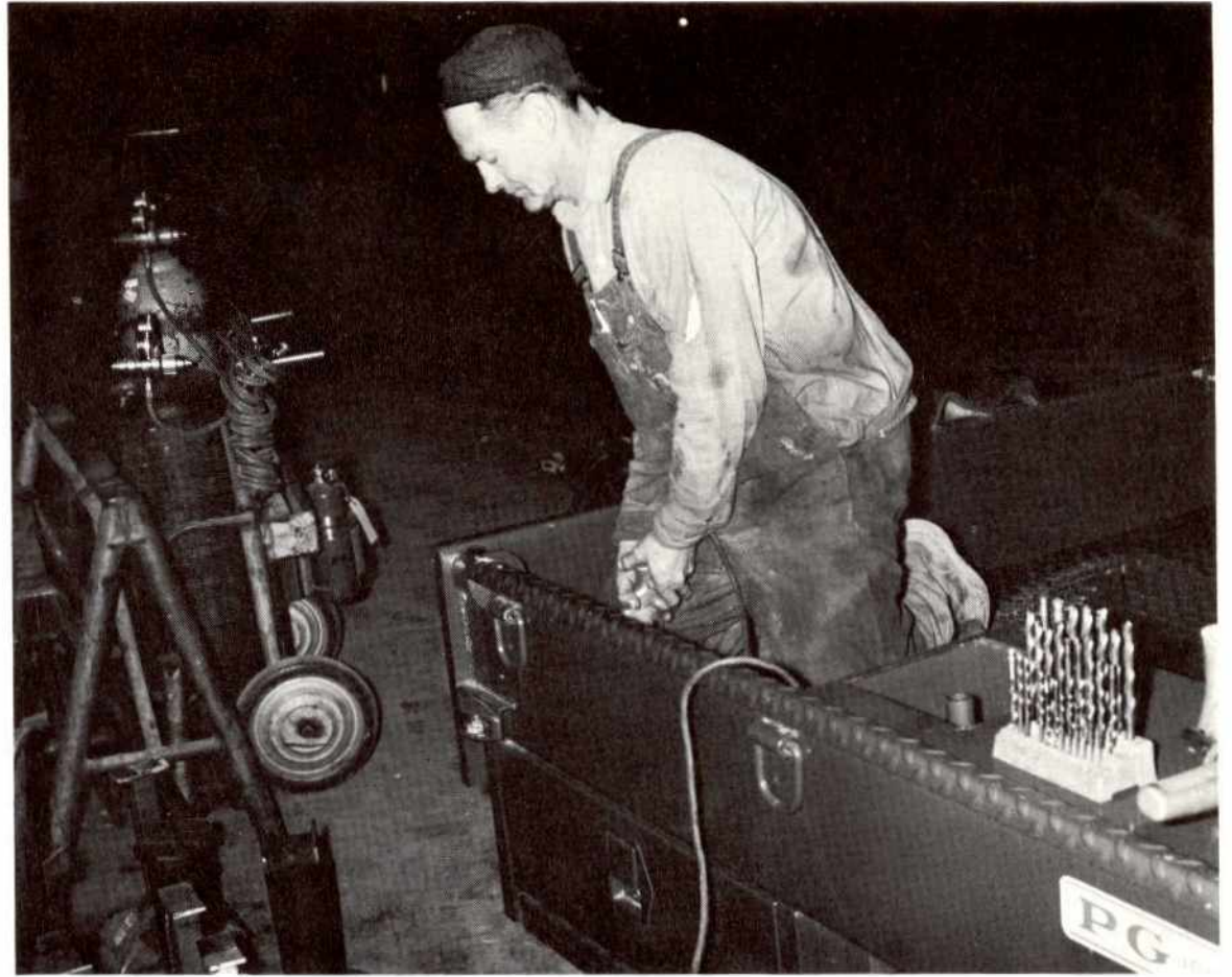
Bob Gubel, a Welder at the Davis Service Center, drills holes in a line truck trailer preparatory to installing boom extension brackets.
