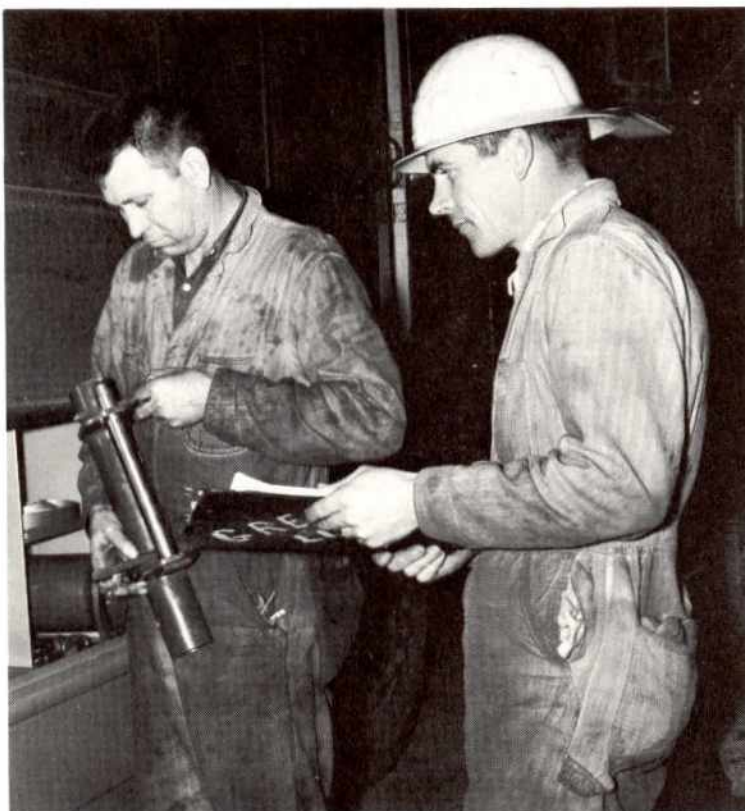
Lee Montgomery, right, and Guy Ross check out a basket extension in the tool locker of a new FWD Tractioneer G.C. line truck being inspected at Davis yard before it goes out into the field. This FWD truck is a new type of 6 wheel drive vehicle used in line construction.
