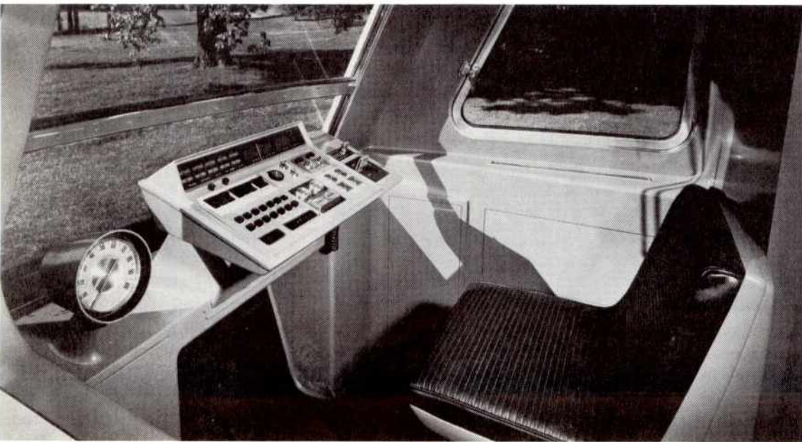
An attendant, sitting in the nose pod of each Bay Area rapid transit train, will monitor performance of the train and, if necessary, will be able to exercise control over the vehicle. Normally all trains will be operated automatically by a central computer.
