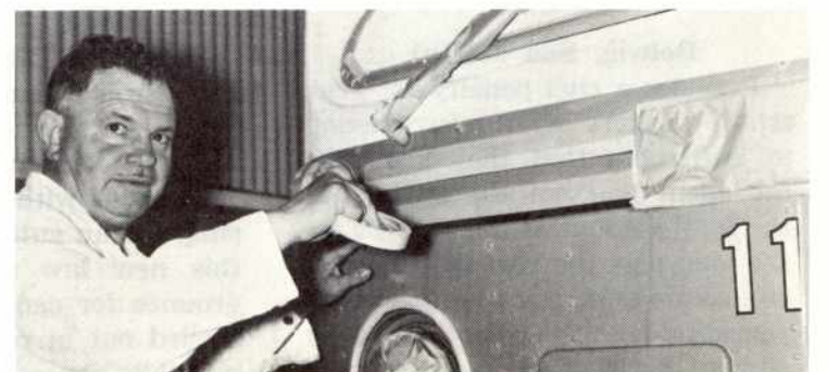
3. Complete paint jobs on STA coaches, including the Christmas Candy Cane bus, are done by Frank Cernicky shown masking the front end of a GM TDH-3610.
