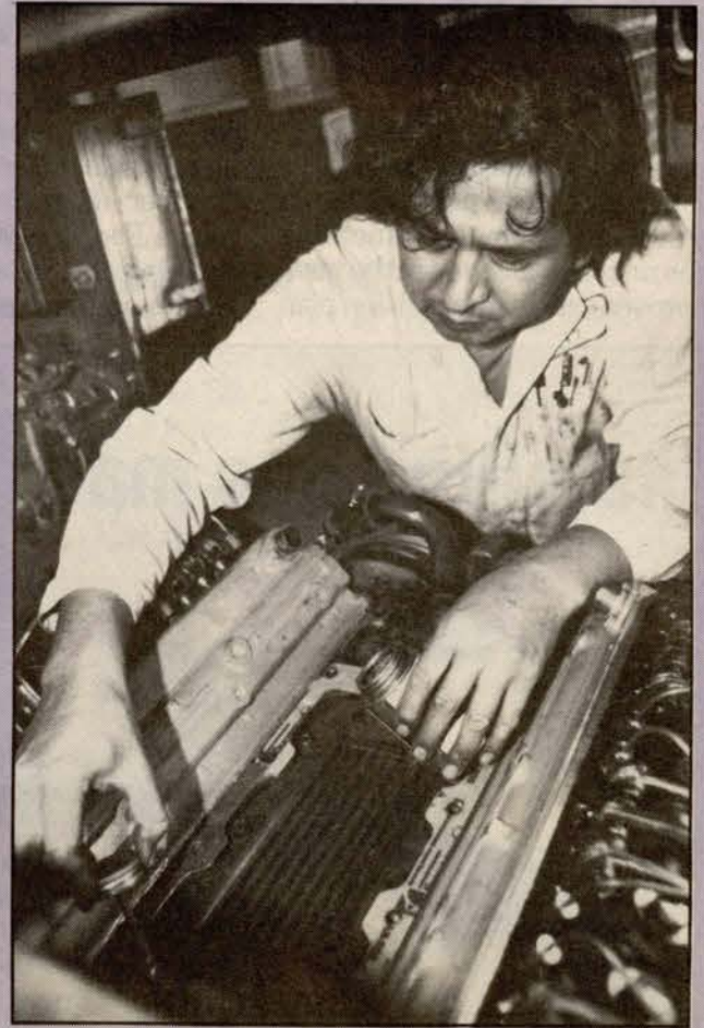
Mondo Lozoya, performing complete in-frame overhaul on Gillig Coach, applies 'Never Seez' to blower gasket.
