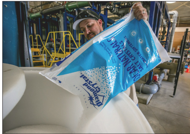
John Sanneman dumps salt into a tank to make chlorine at the water micro-filtration plant.
