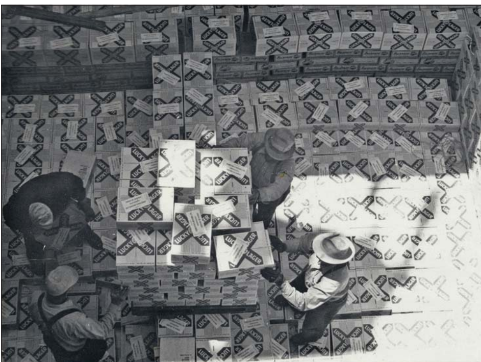
A shipment of beer being handled by a longshore crew in 1956. Such products could be handled more efficiently when they were fastened together in larger units.
