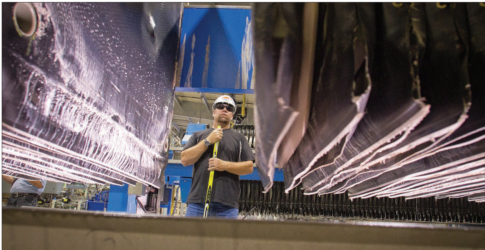
Mark Dempsey, Combustion Turbine Specialist, monitoring a filter press operation.
