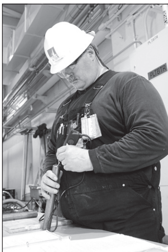
Machinist Kris Evangelo marks studs with heat trace number and material number.
