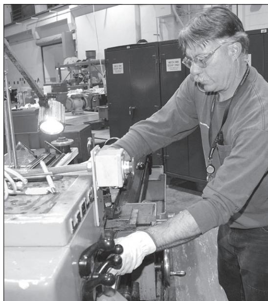
Machinist Dan Ward machines all-thread size length for relief valves.
