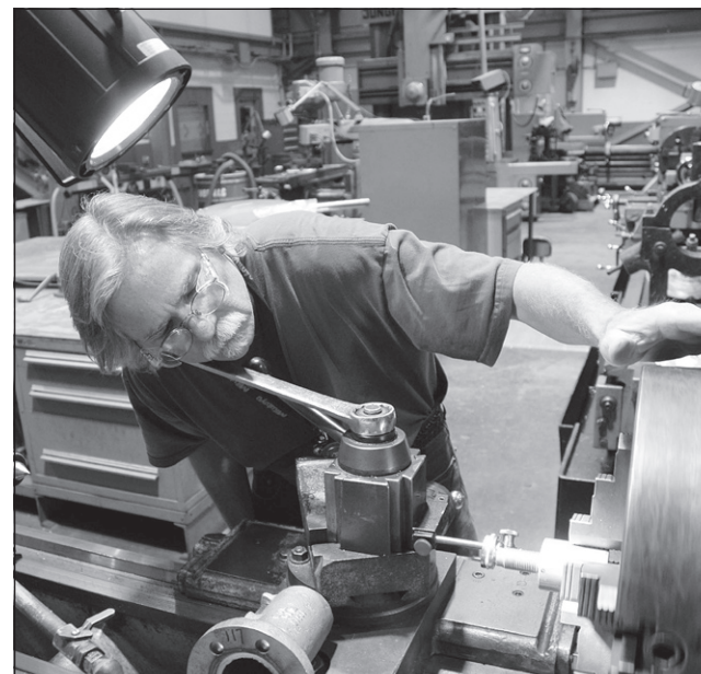
Machinist Subforeman Don Rotta dials in a fixture that's used to hold a valve bonnet to be machined.
