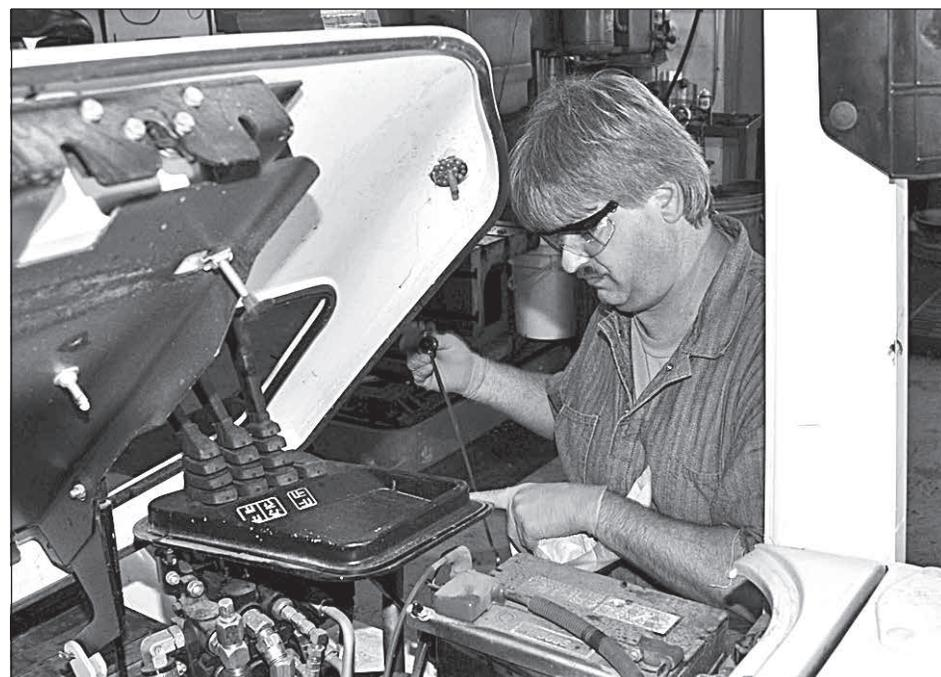
**BELOW: Mechanic/Equipment Operator Kurt Golz services the engine on a fork lift.**
