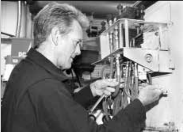
Equipment Mechanic Chris Chapman fixes a leaky control valve on a T-truck aerial lift.
