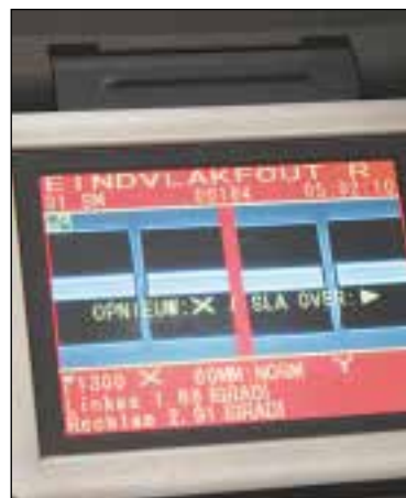
This monitor enables you to watch as the two strands of fiber are brought together in preparation for splicing. Minor adjustments are made automatically to make the fit a perfect one.
