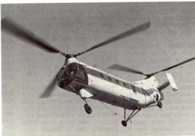
1. An action shot of the "flying banana" used in tower construction on the EHV intertie. The 'copter is based at a heliport 18 miles northeast of Chico. Note the "grab hook" slung from its belly.
